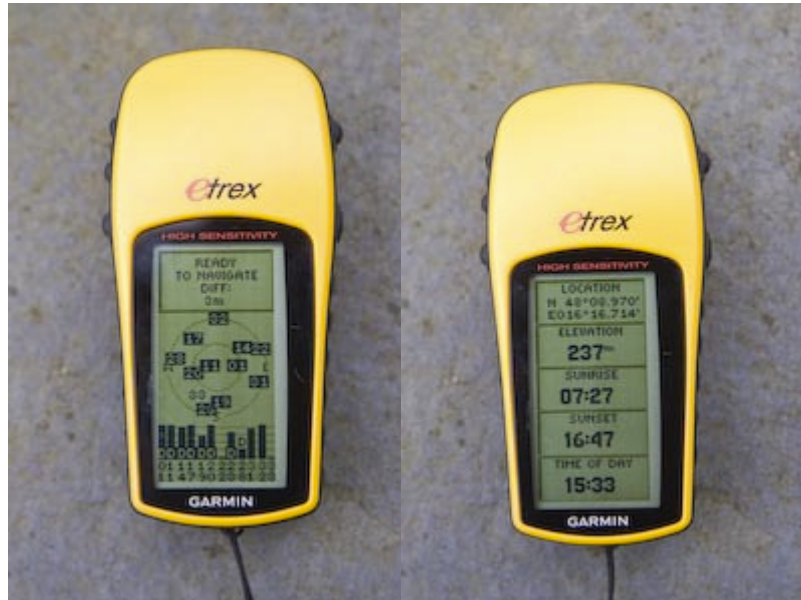
Left: Display showing the satellites received with their respective reception level and satellite numbers. Right, top: Coordinates
