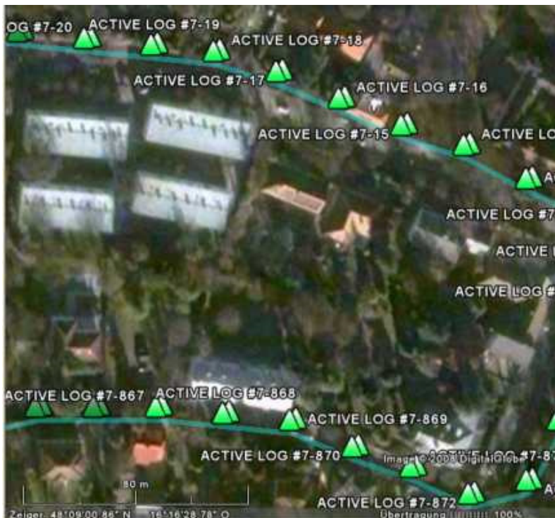
Recorded track data in Google Earth. The recording mode was set to record one track point every 20m (see the scale at the bottom of the picture with a total length of 80m
