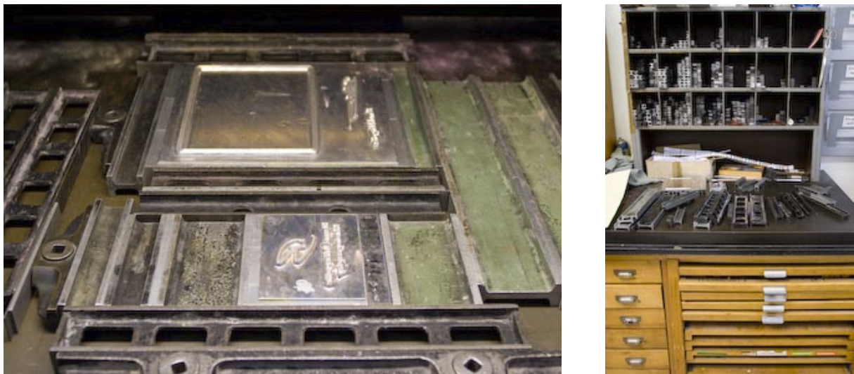
Left: The debossing dye on the mounting plate, Right: Tool required to exactly locate the debossing dye on the mounting plate
