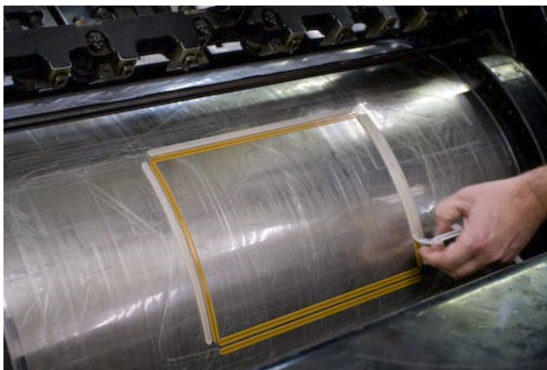
After one run, the complement rails are attached to the revolving unit and the positioning bars can be removed.
